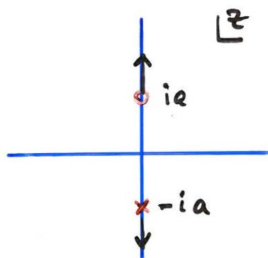
Pole at  $z = -i\alpha$  simple with residue  $\frac{i}{2\pi} \sqrt{a_+ a_-}$
